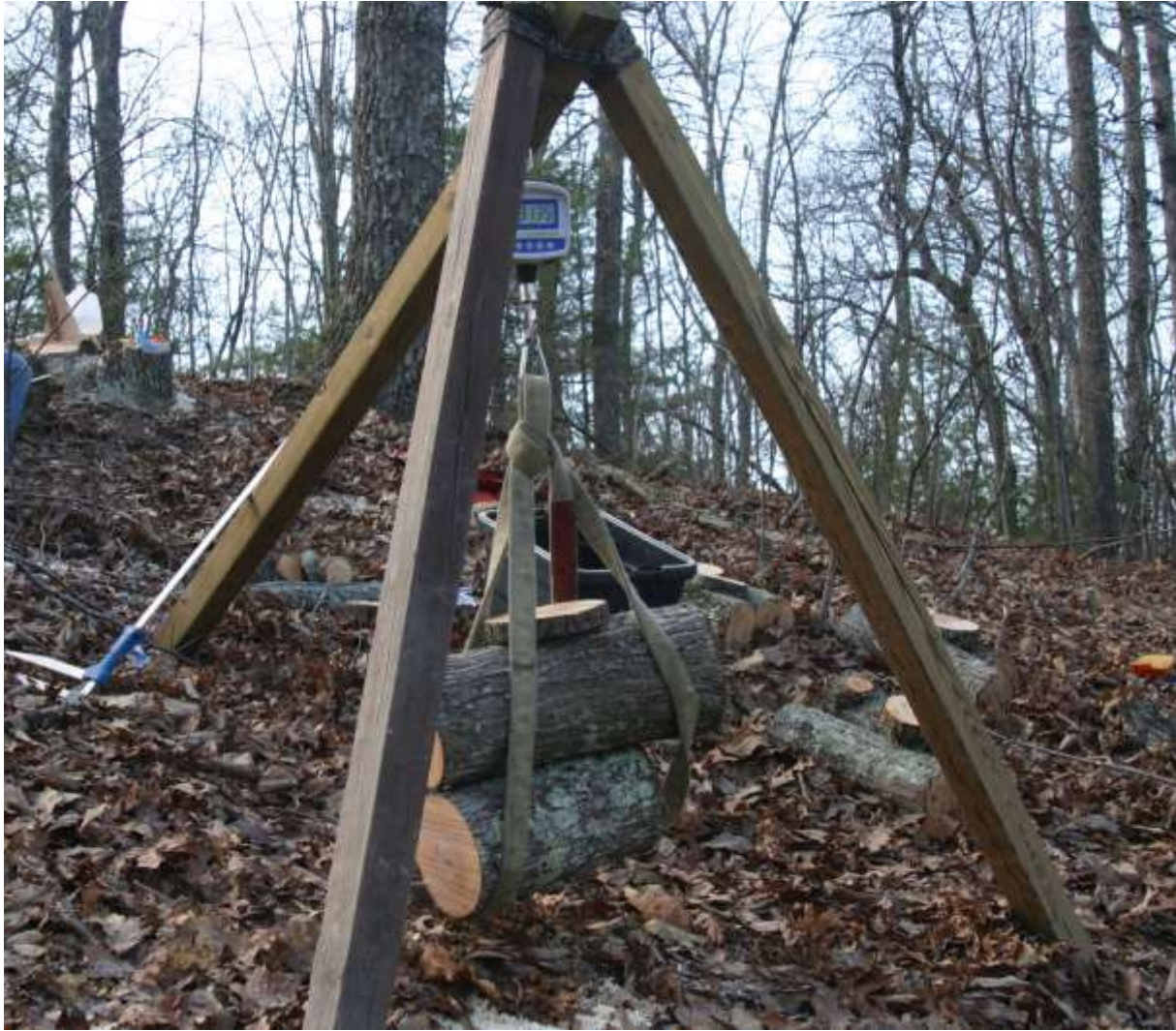
Figure 1. Example of green-weight measurement following cutting of a single disk from a 4' log section. Subtracting the weight of this measurement from the log-section weight made before cutting the disk gives the weight of two sawkerf cuts through the log.
